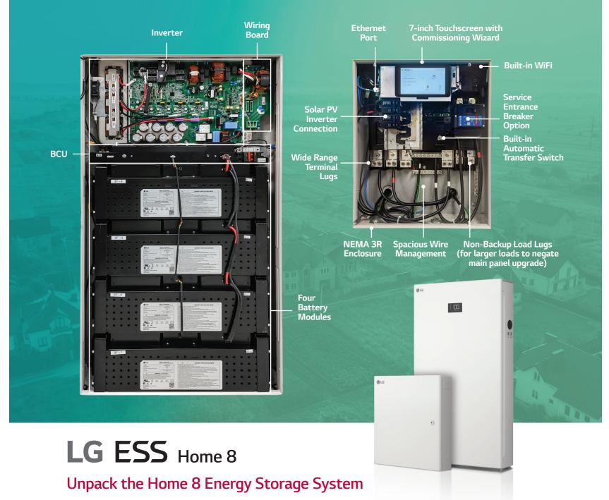
The **LG Electronics Home 8 Energy Storage System** is an all-in-one sustainable energy solution designed with a grid-connected inverter, integrated battery, and innovative Smart Energy Box (SE Box) to protect from outages, rolling blackouts, peak energy shifts, and more.
